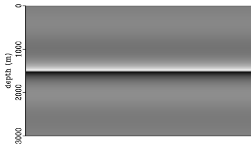
Fig. 10: The new M-OSRP Claerbout III (Stolt extended) migration for 2 way wave propagation. The example with c_0/c_1 velocity. The image both above and beneath the reflector. No "rabbit ears". Consistent image along the reflector. Light color image from above. Dark color image from below. (Qiang Fu and Weglein, 2015)
